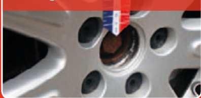
Missing wheel hub trim
